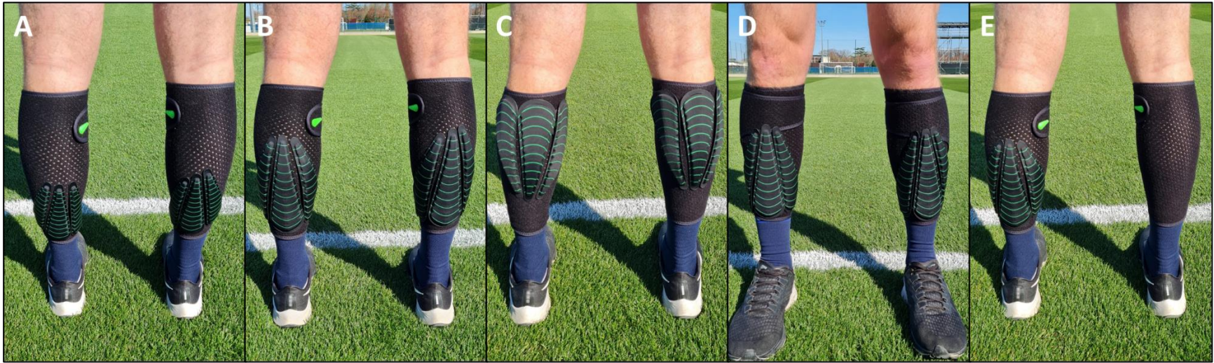
Figure 1. The experimental conditions – WR lower limb loading patterns. Pictures from left to right: A) 0.75% BM distal, posterior loading; B) 1.5% BM distal, posterior loading; C) 1.5% BM proximal, posterior loading; D) 1.5% BM distal, anterior loading; E) 1.5% BM distal, posterior, unilateral loading.
