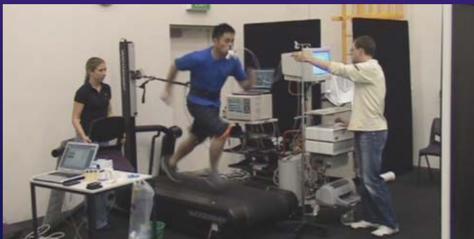
Fig 1. Participant performing a 4-s sprint on the non-motorized treadmill (Force model, Woodway, Waukesha, WI, USA).
